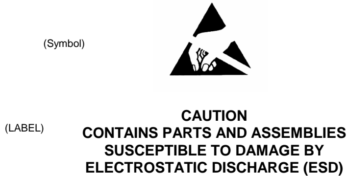
FIGURE 17. Electrostatic discharge (ESD) sensitive identification.
