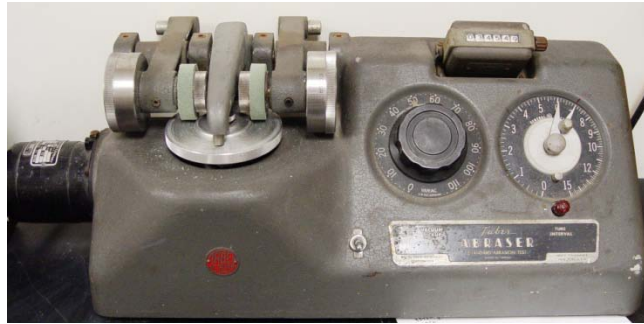
Figure 5. The Taber abraser. Revolution counter (top right), vacuum suction control, and timer seen on right hand side of instrument. Two metallic weights, two green abrasive wheels, vacuum suction arm and metal rotating plate seen on left hand side of instrument. Test plates are bolted to the rotating plate and the green abrasive wheels are off center so they drag/skid/rotate as the test plate rotates beneath them.
