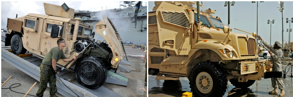
Figure 5. Views of a military wash rack in action.
